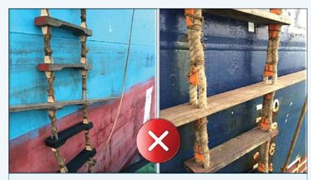
Steps should be horizontal and equally spaced. [2] [8]
