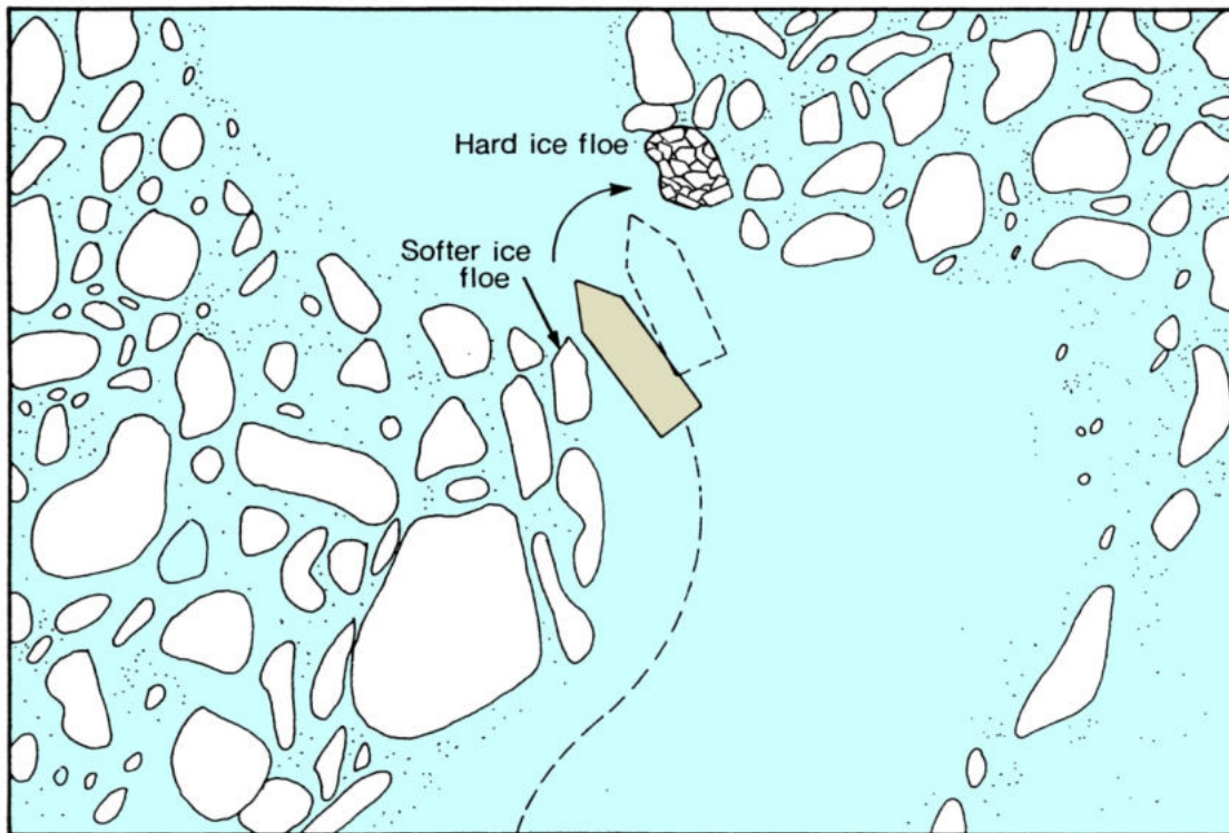
Figure 50: Danger in Turning in an Ice Channel
