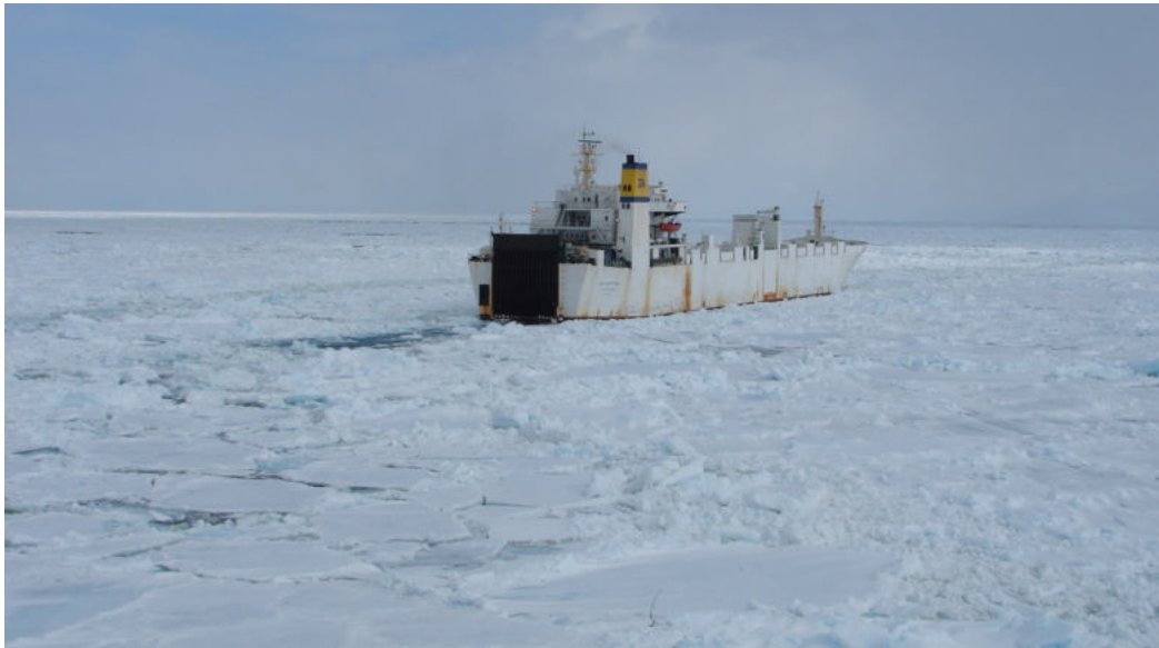
Figure 53: Ice under pressure will close the track behind the vessel
