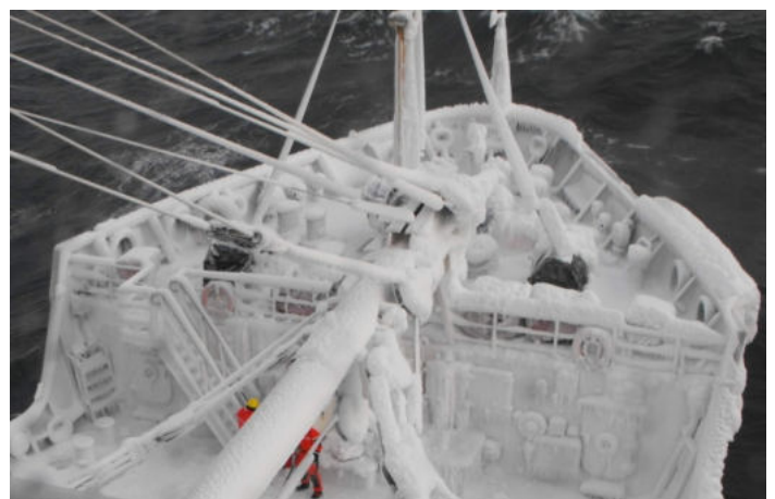
Figure 46: Ice build-up on forecandle
